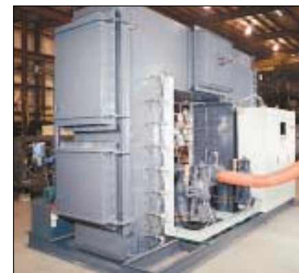
Norbord conducted an extensive 14-month pilot test, pairing an RTO with its EFB system. In 2003, MEGTEC Systems designed and constructed this 1,000 cfm RTO pilot unit and installed it at the discharge of the existing EFB systems at the Bemidji facility. The EFB systems were originally installed in the mid-1980s, designed with only 12-inch-deep filter beds and reaching the end of their useful life. If the RTO pilot revealed promising results, Norbord planned to upgrade to a more advanced EFB system for the final full-scale system. Success of the pilot study led to EFB system upgrades that included 24-inch deep filter beds, a new ionizer design with an advanced automated cleaning system, and improved maintenance features.
