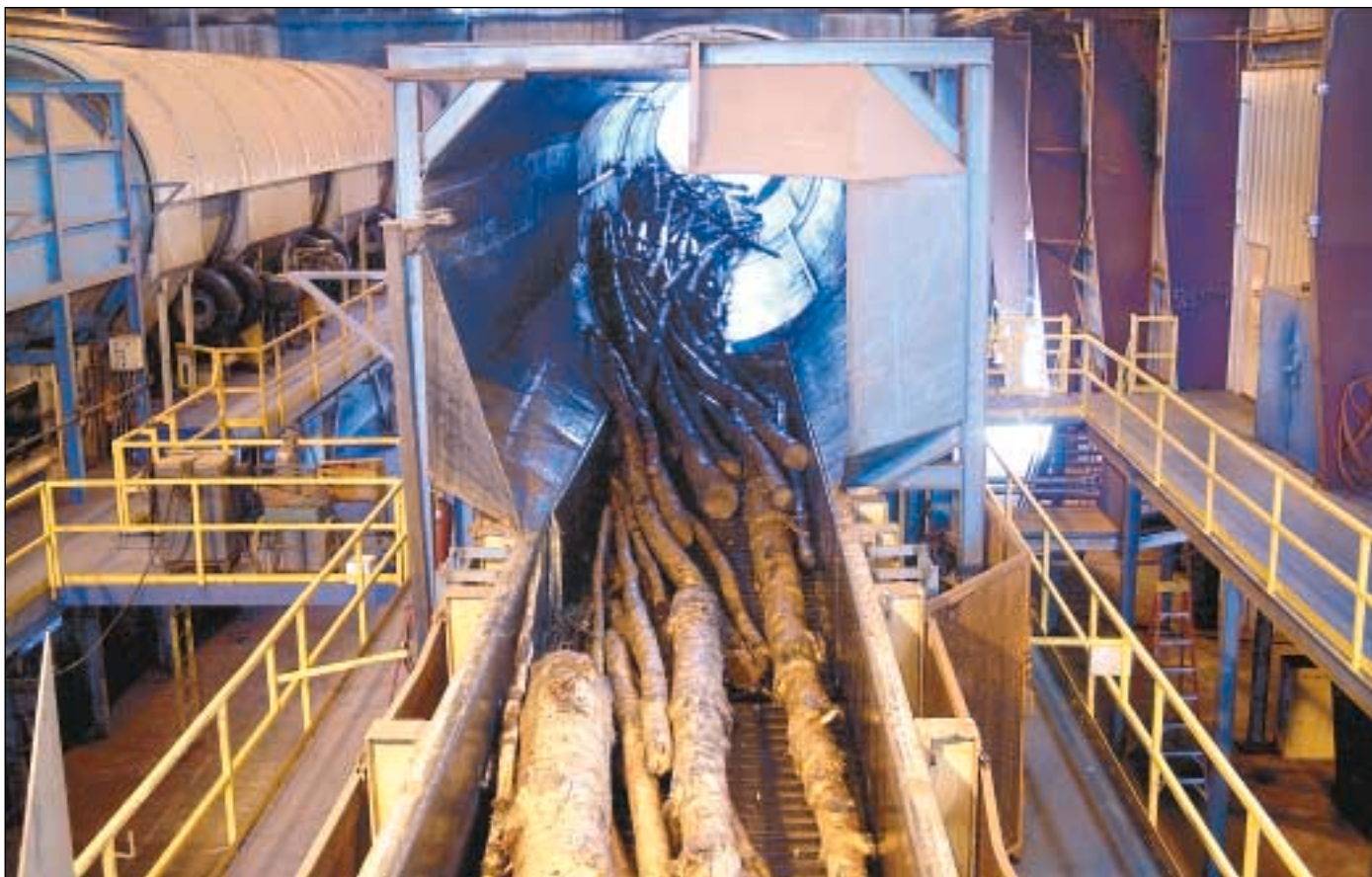
Southern pine logs move through drum debarker.
