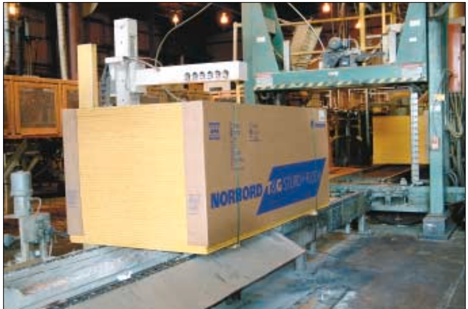
Norbord T&G Sturd-I-Floor is strapped at Signode station.
